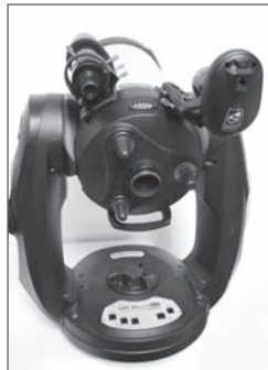
Finder and StarSense installed on CPC 800
