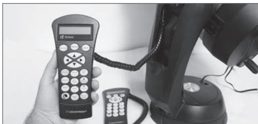
NexStar Hand Control replaced with StarSense Hand Control
