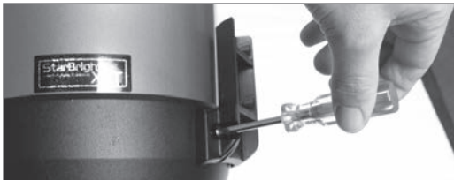
Installing base with Phillips screwdriver
