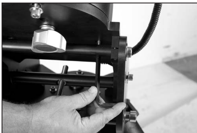
Figure L. Use the provided hex wrench to secure the three 3/8" hex screws into the telescope drive base.
