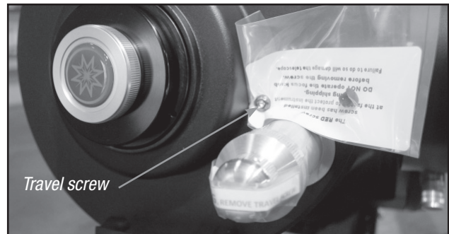
Figure H. Remove the travel screw before operating the focuser. Return the travel screw before shipping the telescope.
