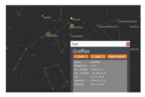
The telescope's current position is indicated by the green crosshair in the SkyViewer. Slewing the telescope in CPWI will move the green crosshair in real time as you slew. When you make a selection in the SkyViewer, a yellow crosshair will appear over the object.
